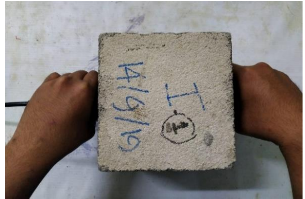
Fig. 2 Direct mehode of UPV test
