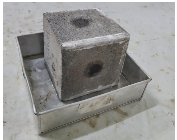
Fig. 3 Initial Rate of Water Absorption (IRA) test
